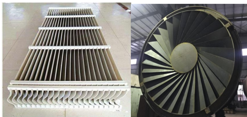
Figure 4. Conventional louver demister (left) and new cyclone demister (right).
